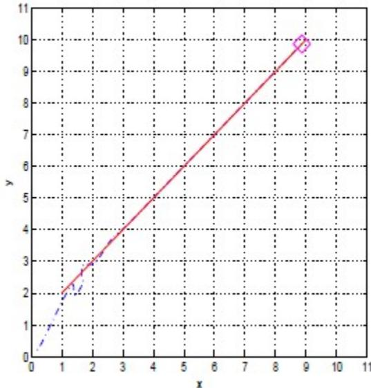
**Reference path 1:** Trajectory tracking for states  $x, y$  of the underactuated hovercraft
