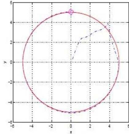
**Reference path 2:** Trajectory tracking for states  $x, y$  of the underactuated hovercraft
