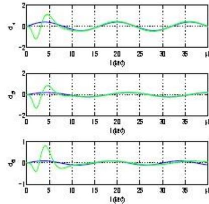
(b) State variables associated with the rotational motion of the AUV
