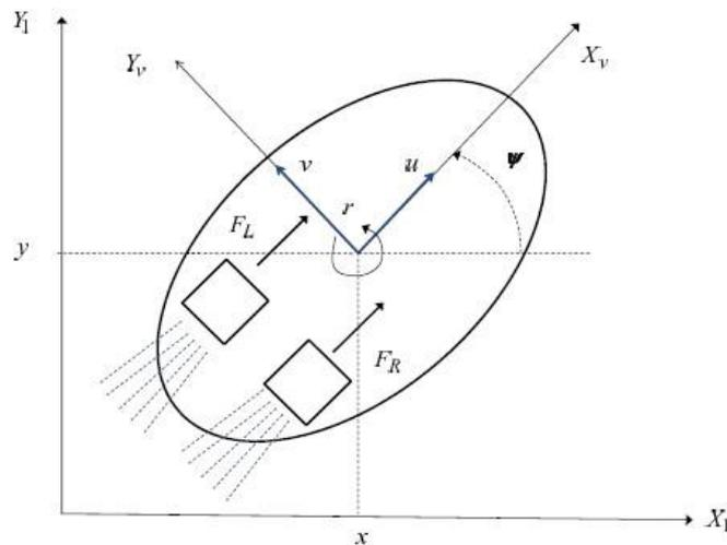
Fig. 1. Diagram of the underactuated hovercraft's kinematic model
