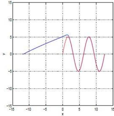
Tracking of the reference trajectory (red line) in the  $x - y$  plane by the unmanned surface vessel (blue line),
