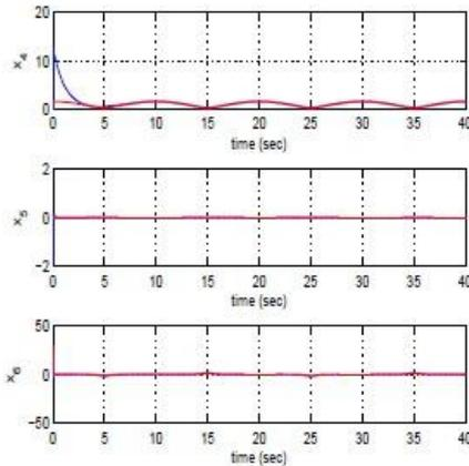
Convergence of the state variables of the vessel  $x_4 = u$ ,  $x_5 = v$  and  $x_6 = r$  to the reference values
