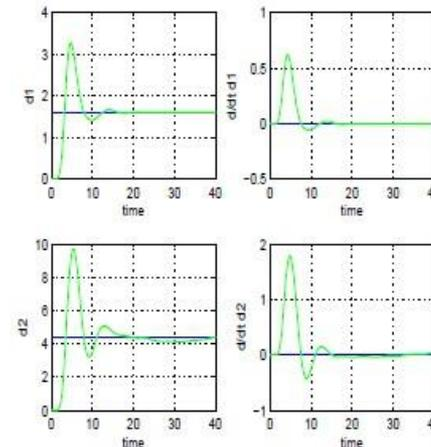
**Reference path 5:** Estimation of disturbance inputs using the Derivative-free non-linear Kalman Filter
