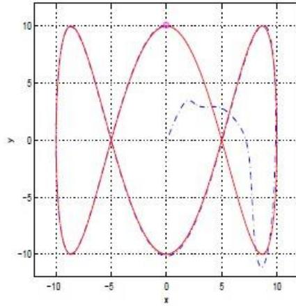
**Reference path 4:** Trajectory tracking for states  $x, y$  of the underactuated hovercraft
