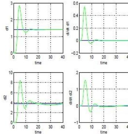
**Reference path 4:** Estimation of disturbance inputs using the Derivative-free non-linear Kalman Filter
