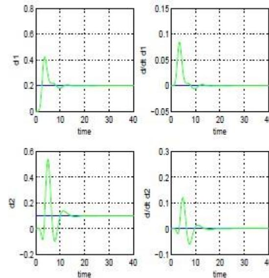
**Reference path 1:** Estimation of disturbance inputs using the Derivative-free non-linear Kalman Filter
