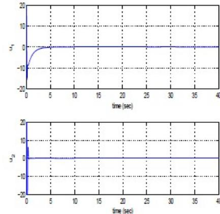
Control inputs  $u_1$  and  $u_2$  exerted on vessel
