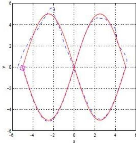
**Reference path 3:** Trajectory tracking for states  $x, y$  of the underactuated hovercraft
