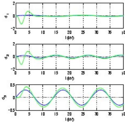
(a) State variables associated with linear motion of the AUV
