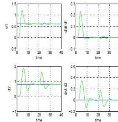
**Reference path 3:** Estimation of disturbance inputs using the Derivative-free non-linear Kalman Filter <sup>30</sup>
