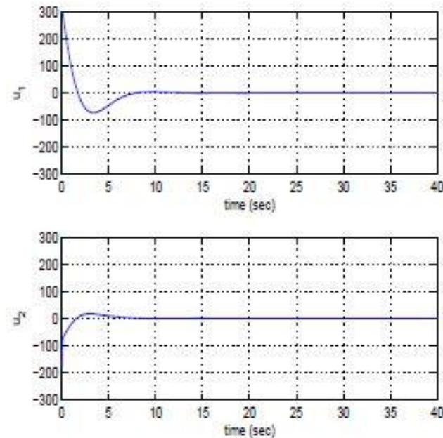
**Tracking of setpoint 3:** (b) variation of the submarine's control inputs
