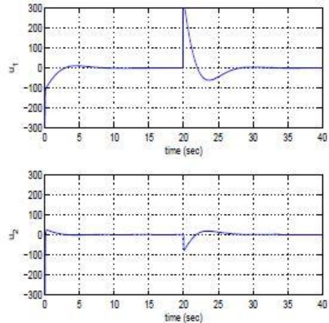
**Tracking of setpoint 5:** (b) variation of the submarine's control inputs
