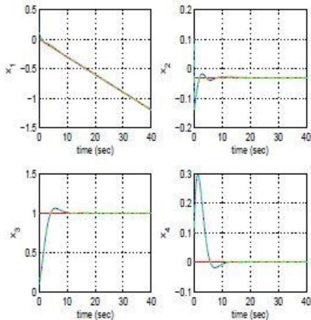
**Tracking of setpoint 3:** (a) Convergence of the state variables (blue lines) to setpoints (red lines) and their state estimates (green lines)
