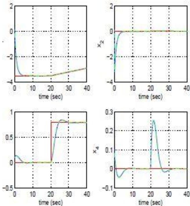
**Tracking of setpoint 5:** (a) Convergence of the state variables (blue lines) to setpoints (red lines) and their state estimates (green lines)
