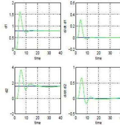
**Reference path 2:** Estimation of disturbance inputs using the Derivative-free non-linear Kalman Filter
