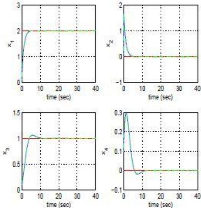
**Tracking of setpoint 1:** (a) Convergence of the state variables (blue lines) to setpoints (red lines) and their state estimates (green lines)
