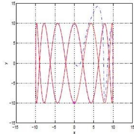
**Reference path 5:** Trajectory tracking for states  $x, y$  of the underactuated hovercraft
